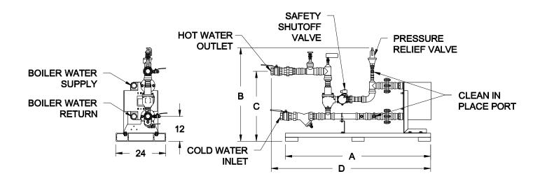
4 gpm minimum recirculation flow through EZ Plate required. All dimensions are in inches.
