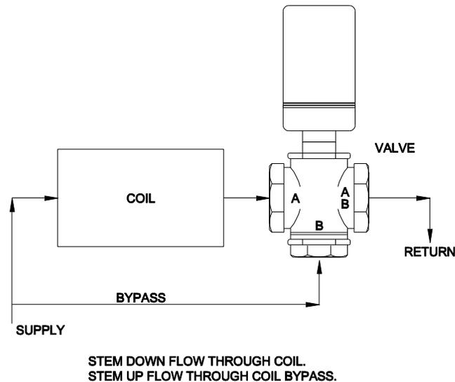
3. When the demand is satisfied, the limit operating circuit opens and the valve actuator is de-energized. The actuator motor stops running and the actuator shaft spring returns to the diverting position causing the boiler water to divert through the bypass ports and return to the boiler water supply loop.
