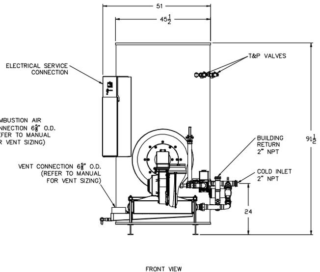
Recommended Service Clearance: 18" from all sides, 12" from the top. Consult factory for heat exchanger pull space requirements.
