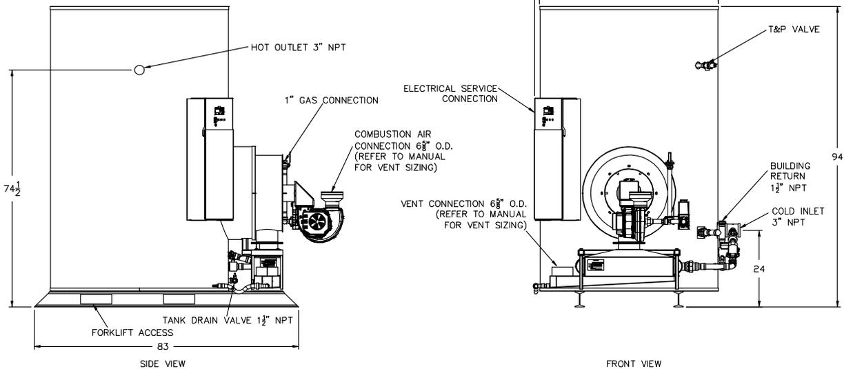
Recommended Service Clearance: 18" from all sides, 12" from the top. Consult factory for heat exchanger pull space requirements.
