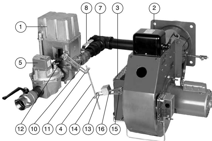
**MECHANICAL OPERATION:** The Low-High-Off system uses a Motorized Gas Valve (1) to control the Low-High-Off operation of gas to the Blast Tube (2), as well as
