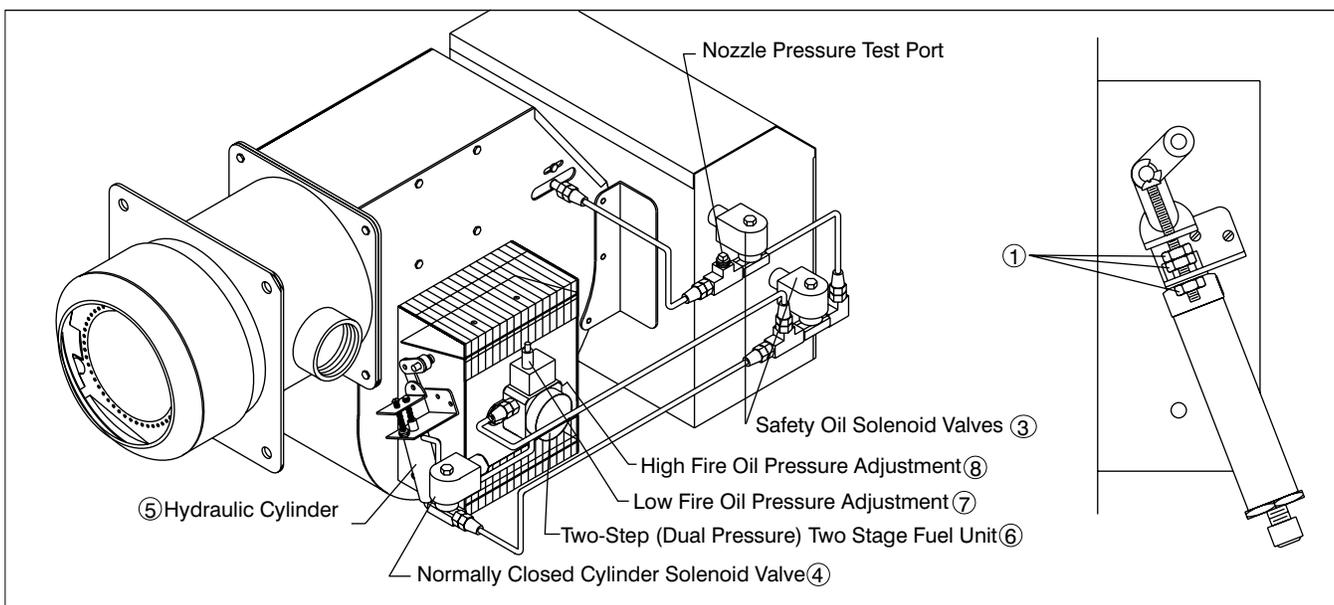
**MECHANICAL OPERATION:** The RALFS system uses a two step, two stage dual pressure Oil Pump (6), or fuel unit, with a simplex nozzle. Either a direct spark or a gas pilot ignition system may be provided for ignition of the main oil flame. The air damper is spring loaded to an open position suitable for maximum desired capacity and proper combustion.
