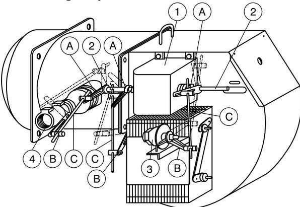
Typical general linkage arrangement for combination gas/oil full modulation burner, shown in low fire light off position. Dotted lines indicate approximately high fire position. When making adjustments, make certain the motor can make its full 90° stroke without any linkage binding.
