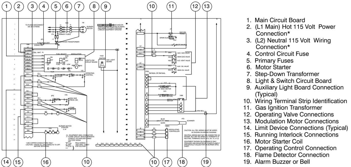
\* L1 Main 115 volt hot incoming power terminal is located at the top of the circuit board. L2 Neutral 115 volt power terminal is located on the lower set of terminals at the bottom of the main circuit board. The L1 Fused terminal (not shown) located on the lower set of terminals is for factory use and should not be used for incoming power connections.
