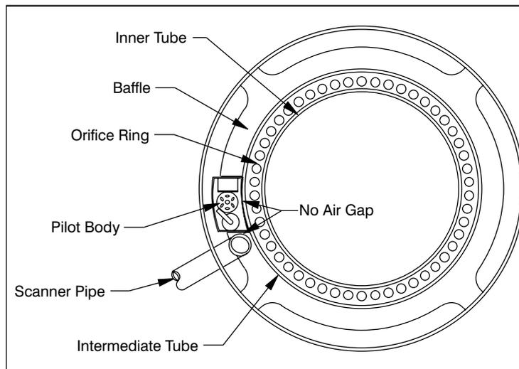
Pilot case to gas manifold adjustment is very important. As depicted, the inside radius of the pilot body must be tight against the outside radius of the gas manifold.
