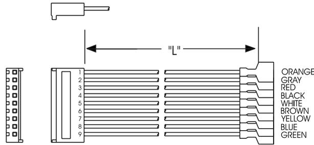
To make a harness select Amp connector housing Part Number 770849-9 and Amp housing terminal Part Number 770552-1
