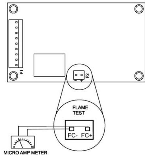
Flame current is the current that passes through the flame from the sensor to ground. The minimum flame current necessary to keep the system from lockout is 1.0 microamps. To measure flame current, connect an analog DC microammeter to the FC terminals per Figure 5. Meter should read 1.0 mA or higher. If meter reads below "0" on scale, meter leads are reversed. Disconnect power and reconnect meter leads for proper polarity.
