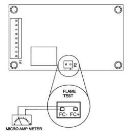
Flame current is the current that passes through the flame from the sensor to ground. The minimum flame current necessary to keep the system from lockout is 1.0 microamps. To measure flame current, connect an analog DC microammeter to the FC terminals per Figure 5. Meter should read 1.0 mAor higher. If meter reads below "0" on scale, meter leads are reversed. Disconnect power and reconnect meter leads for proper polarity.
