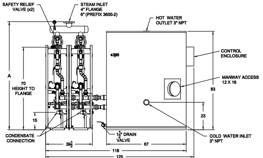
Completed piping assembly is factory fit between the exchanger and tank and is separated at unions for shipping.
