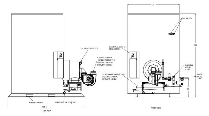
Recommended Service Clearance: 18" from all sides, 12" from the top. Consult factory for heat exchanger pull space requirements.
