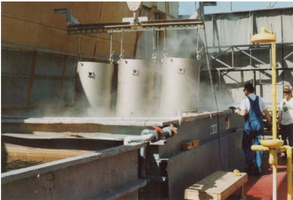
Three vertical tube water heater tanks are withdrawn from the electroless nickel plating bath.
