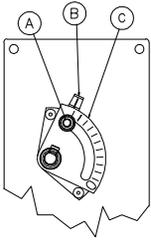
Loosen the locking screw (A) and move the lever (B) along the scale (C) to the position wanted and tighten the screw. Check the air adjustment by making a flue gas analysis.
