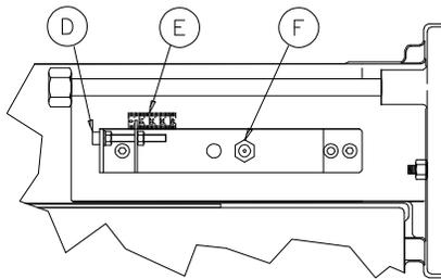
High carbon monoxide can be caused by a misaligned gas nozzle assembly. Turning the adjustment screw (D) clockwise will retract the gas nozzle assembly, which can improve alignment.
