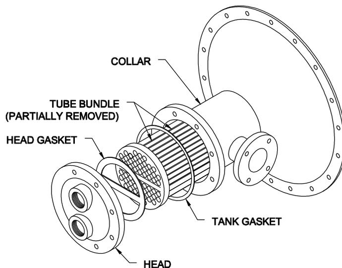
4. When replacing the heat exchanger HEAD, use a calibrated torque wrench to tighten the bolts/studs and nuts in an alternating star pattern. Use the following chart as a guide. All heat exchanger head torque values apply to well-lubricated nut bearing surfaces.
