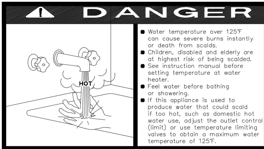
***Thermostatically controlled mixing valves must be used in the design of the potable hot water system.***
