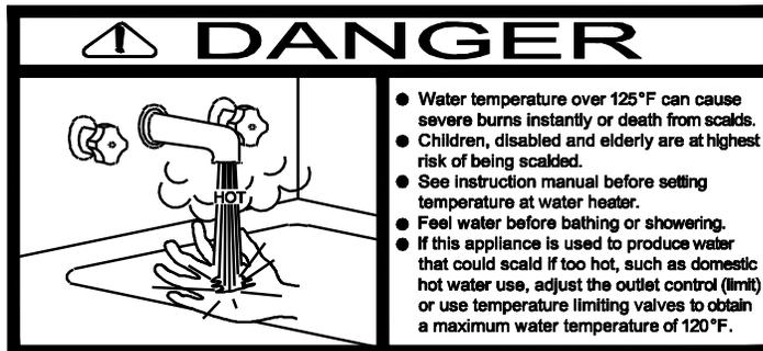
***Thermostatically controlled mixing valves must be used in the design of the potable hot water system. Potable hot water should be tempered to no more than 110°F when used for bathing or other personal uses.***
