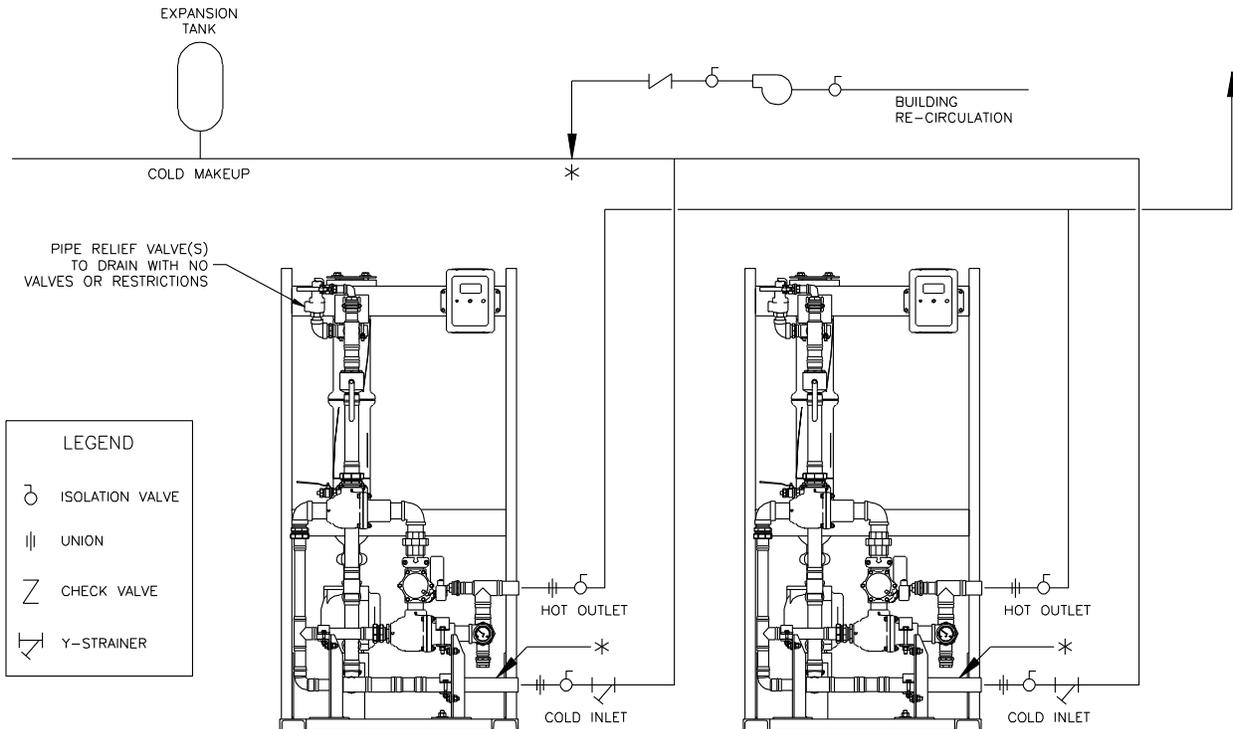
\* Dedicated connection for building recirculation on heaters with optional sub-cooler.
