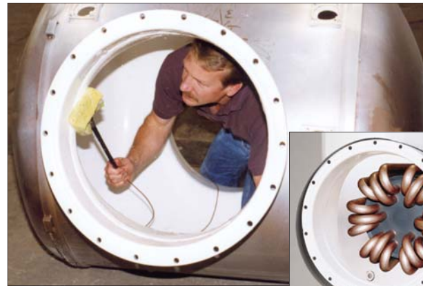
Wet electrode test ensures lining integrity. All TURBOPOWER 99 tanks are tested and all must pass inspection before shipping.
