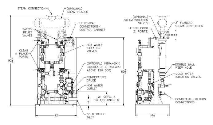
4 gpm minimum recirculation flow through CCX required; can be provided by optional intra-skid circulator. All dimensions are in inches.
