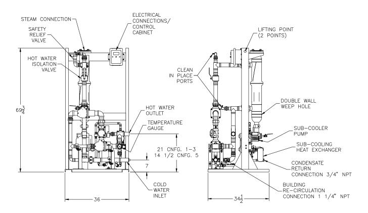
4 gpm minimum recirculation flow through CCX required; can be provided by optional intra-skid circulator.
