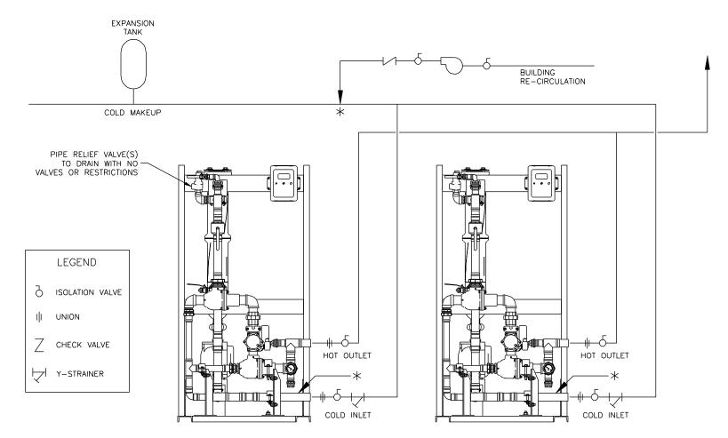
\* Dedicated connection for building recirculation on heaters with optional sub-cooler. Connect recirculation to this point instead of cold inlet if sub-cooler is ordered.
