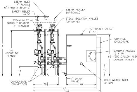
Completed piping assembly is factory fit between the exchanger and tank and is separated at unions for shipping. Tank and heat exchanger ship separately for field connection to piping assembly.
