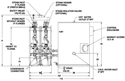
Completed piping assembly is factory fit between the exchanger and tank and is separated at unions for shipping. Tank and heat exchanger ship separately for field connection to piping assembly.
