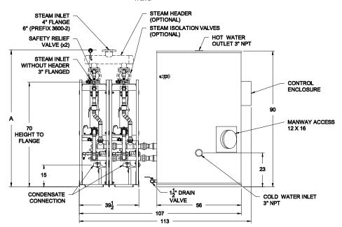
Completed piping assembly is factory fit between the exchanger and tank and is separated at unions for shipping.
