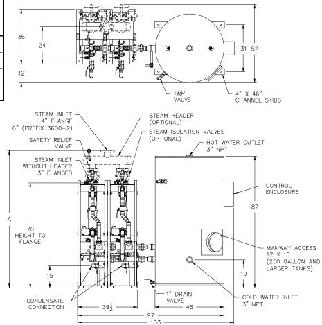
Completed piping assembly is factory fit between the exchanger and tank and is separated at unions for shipping. Tank and heat exchanger ship separately for field connection to piping assembly.
