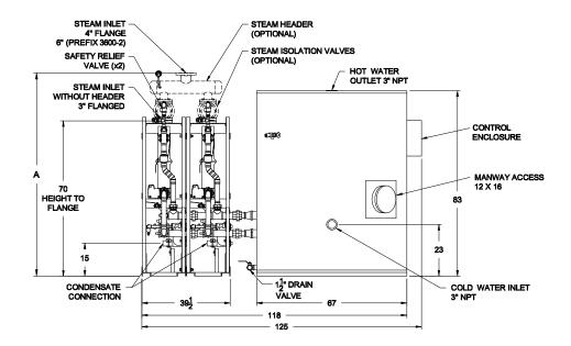
Completed piping assembly is factory fit between the exchanger and tank and is separated at unions for shipping. Tank and heat exchanger ship separately for field connection to piping assembly.
