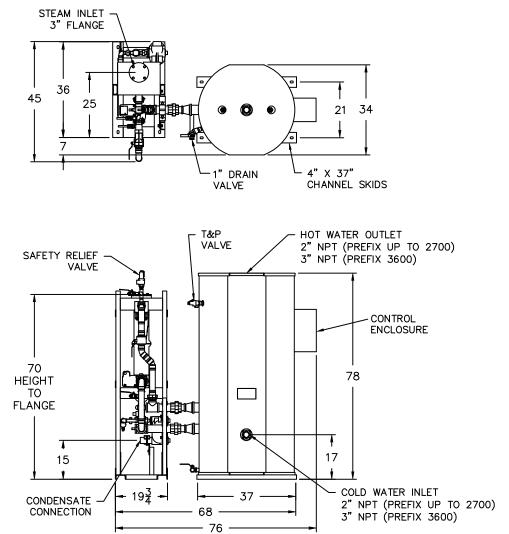
Completed piping assembly is factory fit between the exchanger and tank and is separated at unions for shipping. Tank and heat exchanger ship separately for field connection to piping assembly.
