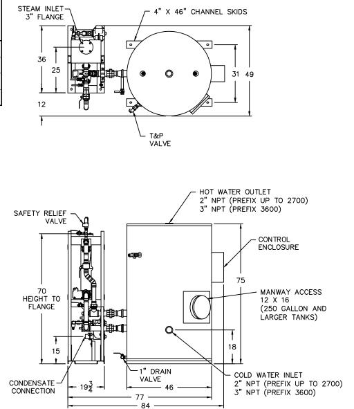
Completed piping assembly is factory fit between the exchanger and tank and is separated at unions for shipping. Tank and heat exchanger ship separately for field connection to piping assembly.
