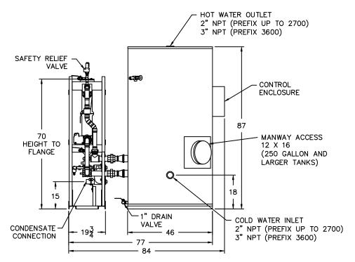
Completed piping assembly is factory fit between the exchanger and tank and is separated at unions for shipping. Tank and heat exchanger ship separately for field connection to piping assembly.
