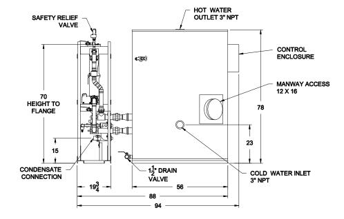
Completed piping assembly is factory fit between the exchanger and tank and is separated at unions for shipping.
