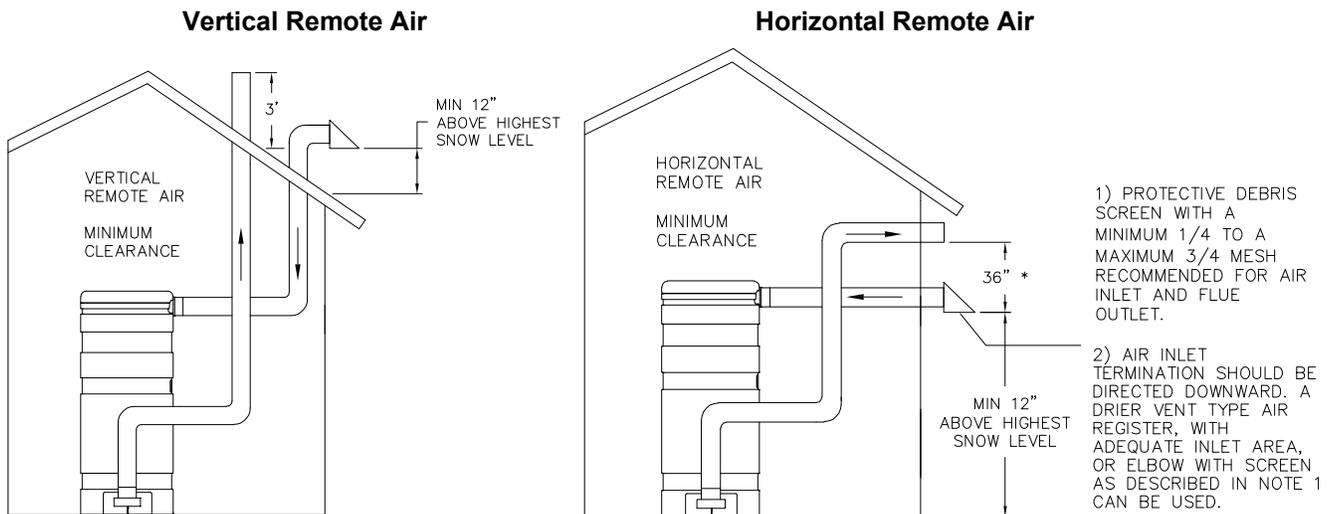
\* When flue outlet is terminated with a straight discharge, separation of terminations must be a minimum of 18".
