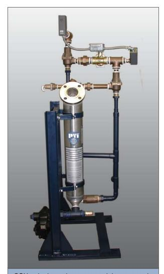
CSX single-exchanger models range in output from 15 to 75 gpm of 140°F water with 15 psi steam. Dual-exchanger models are available. Heaters are fully packaged and require only jobsite connection to steam, condensate return, water and 120VAC service.
