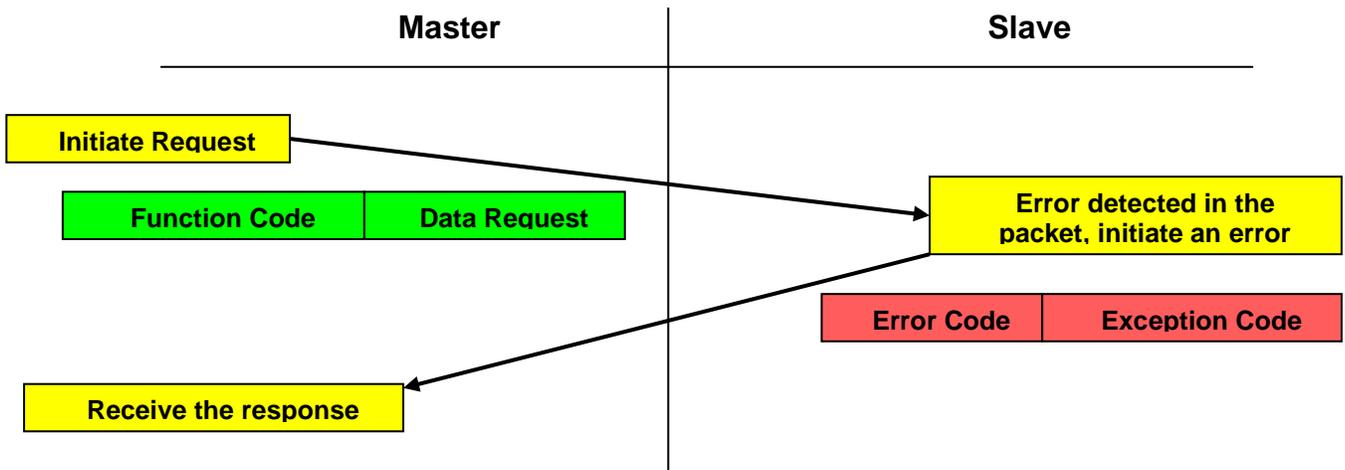
Figure 2 MODBUS Transaction (Error, Exception Code response)
