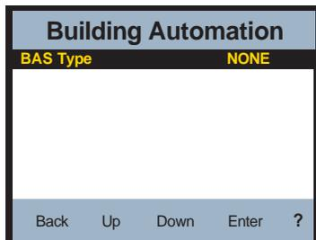
The default “BAS Type” is “NONE” as shown above. To change this setting press the **Enter** icon and the “BAS Type” adjustment screen will appear (as shown below).
