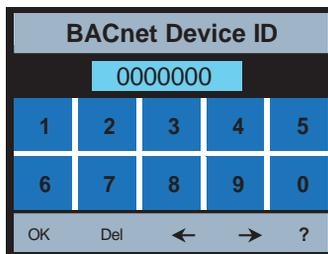
To adjust the ID depress the **Del** key 7 times and enter an ID appropriate for the remainder of the BAS system and press **OK**. Similarly, enter an appropriate “BACnet Port.” To change “Register Foreign Dev” to “ON” scroll down to “Register Foreign Dev” using the **Up** and **Down** icons and select **Enter**. The “Register Foreign Dev” setting adjustment screen is shown in the “OFF” state below.
