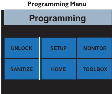
On the "Programming" Menu the **UNLOCK** and **HOME** icons are the only active icons until the control is unlocked. See "Unlock the System" in the "Set up and Programming" section of this Manual.
