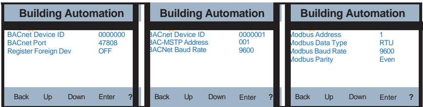
Each of the settings can be adjusted by depressing the **Up** and **Down** icons to highlight the setting of interest and depressing the **Enter** icon to adjust the setting.
