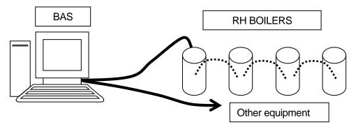
Building Automation System (BAS) connecting directly to MASTER boiler using twisted pair wire. (Wiring is RS-485 physical layer.) MASTER boiler is connected to MEMBER boiler through a special CASCADE wiring. In this configuration, the BAS will get all information for the entire boiler group from the MASTER boiler.
