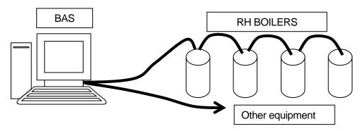
Building Automation System (BAS) connecting directly to each boiler using twisted pair wire. (Wiring is RS-485 physical layer.) This is used when the CASCADE group control feature is not to be used, and the BAS intended to control each boiler individually. Common in 1 and 2 boiler configurations.
