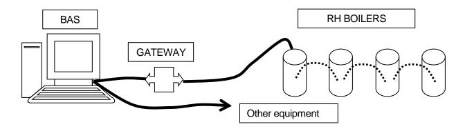
Building Automation System (BAS) connecting to a  $3^{RD}$  party gateway. This can provide interface to building automation system running other protocols. In order to interface with our boilers, the gateway will need to address our boilers using MODBUS RTU or BACNET MSTP
