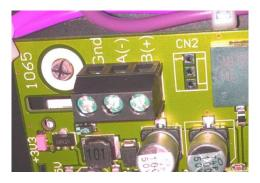
The RS-485 PORT: Both MODBUS RTU and BACNET MSTP connect to this port, selecting the protocol is done in the settings on the display.
