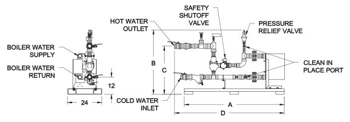
4 gpm minimum recirculation flow through EZ Plate required. All dimensions are in inches.
