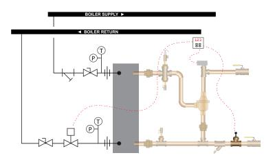
Note: The piping illustrations are generalized. When applying low-water-volume instantaneous water heaters such as EZ Plate, there are additional considerations for the boiler loop. Characteristics such as boiler loop water volume, the number and type of boilers and the energy requirements of the domestic water system relative to the total boiler system BTU output must be taken into consideration. Contact with your PVI representative for design assistance.
