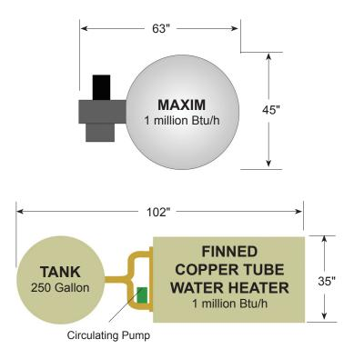
Less Floor Space - depending upon input, the amount of floor space occupied by Maxim is from 20% to 50% less than the typical boilerand-tank water heater.
