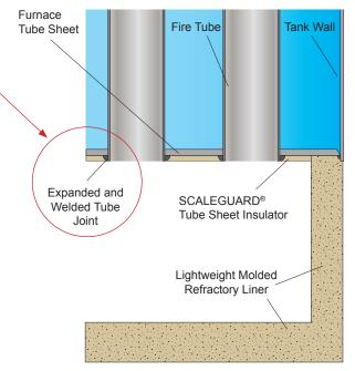
Detail of MAXIM Combustion Chamber and Tube Sheet Construction
