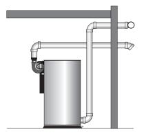
Sealed combustion with sidewall terminations
