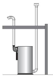
Sealed combustion with roof terminations
