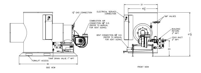
Recommended Service Clearance: 18" from all sides, 12" from the top. Consult factory for heat exchanger pull space requirements. Minimum Clearances: 6" from all sides and top, 24" from the front.
