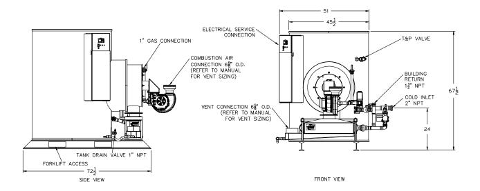
Recommended Service Clearance: 18" from all sides, 12" from the top. Consult factory for heat exchanger pull space requirements. Minimum Clearances: 6" from all sides and top, 24" from the front.
