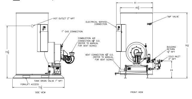
Recommended Service Clearance: 18" from all sides, 12" from the top. Consult factory for heat exchanger pull space requirements. Minimum Clearances: 6" from all sides and top, 24" from the front.
