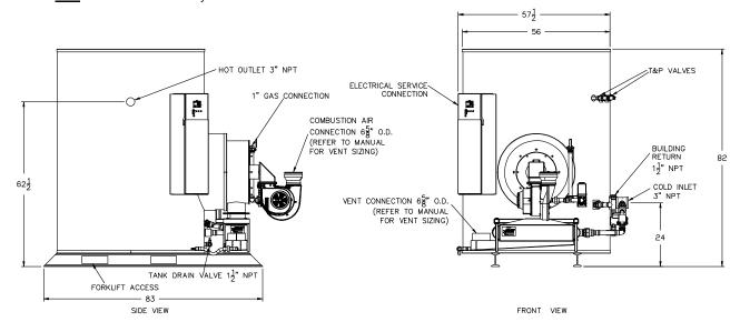
Recommended Service Clearance: 18" from all sides, 12" from the top. Consult factory for heat exchanger pull space requirements. Minimum Clearances: 6" from all sides and top, 24" from the front.
