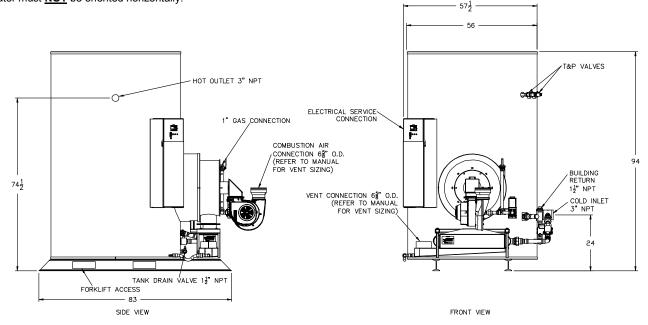
Recommended Service Clearance: 18" from all sides, 12" from the top. Consult factory for heat exchanger pull space requirements. Minimum Clearances: 6" from all sides and top, 24" from the front.
