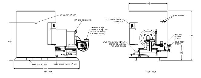
Recommended Service Clearance: 18" from all sides, 12" from the top. Consult factory for heat exchanger pull space requirements. Minimum Clearances: 6" from all sides and top, 24" from the front.
