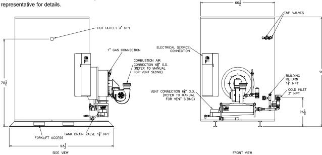
Recommended Service Clearance: 18" from all sides, 12" from the top. Consult factory for heat exchanger pull space requirements. Minimum Clearances: 6" from all sides and top, 24" from the front.
