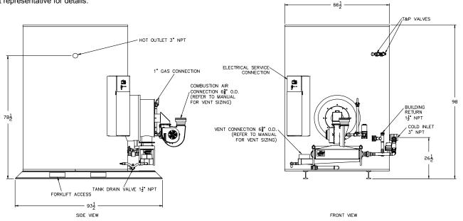
Recommended Service Clearance: 18" from all sides, 12" from the top. Consult factory for heat exchanger pull space requirements. Minimum Clearances: 6" from all sides and top, 24" from the top.
