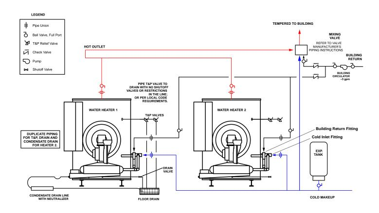
Size common piping for the maximum anticipated flow at a velocity of no greater than 6 feet per second. Type L copper pipe is recommended. Condensate line can be PVC. Refer to PVI installation manual for complete details.
