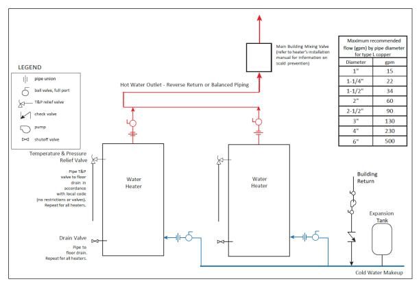
Two Water Heaters - Single Hot Outlet Temperature
