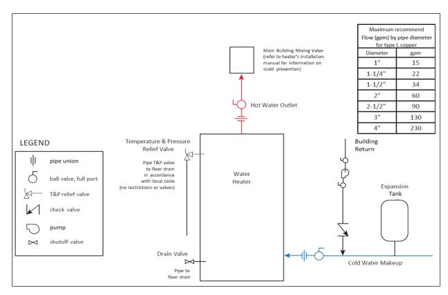
Single Water Heater - One Hot Outlet Temperature
