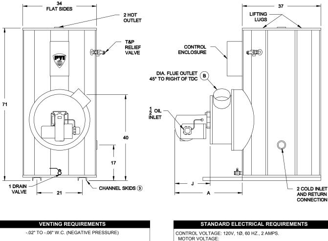
ENTIRE VENT SYSTEM SHOULD NEVER BE SIZED BASED UPON THE VENT CONNECTION DIAMETER EXCLUSIVELY. FOR PROPER SIZING, CONSULT VENTING SUPPLIER.
