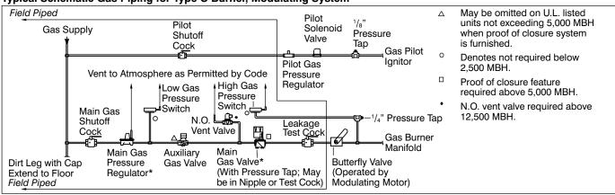
\* On some burner models at inputs below 2500 MBH a combination pressure regulator/automatic gas valve may be used in place of the separate main gas pressure regulator and main gas shutoff valve shown in Figure 8 and 9 above. For specifics on your burner refer to the gas piping diagram supplied with the burner.
