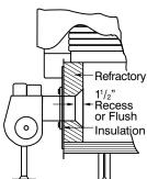
Note: The above minimum dimensions are recommended. If boiler dimensions are less, consult with factory. All burners set through refractory with sleeve to allow field removal. Unlined space between sleeve and burner blast tube closed with non-asbestos high-temp rope or KA-O-Wool.
