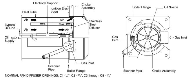
JOB CONDITIONS such as high altitude may require adjustment of diffuser blades to alternate settings. Certain OEM applications may require settings of diffuser blades or electrodes not listed or shown. Setting of electrodes closer to center of nozzle and or farther forward may be required.
