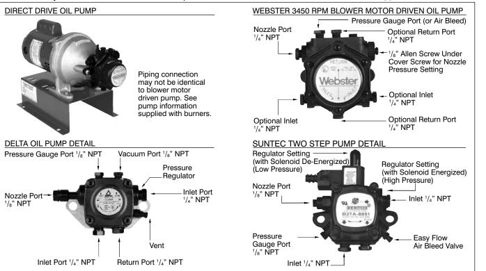
such as the Suntec Model J or H, refer to the pump manufacturer's bulletin that is supplied with the burner.
