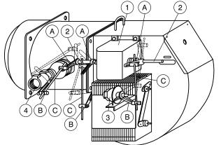
moving it forward decreases the premix air. Generally, the best (quietest/smoothest) operation is in the full forward position with minimum premix air. The premix adjustment is set at the factory in the full forward position. To attain the best combustion results for specific job conditions, change position in small increments.
