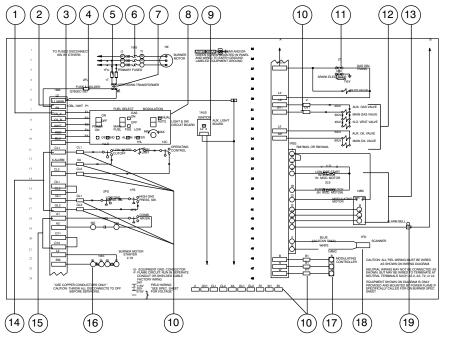
\* L1 Main 115 volt hot incoming power terminal is located at the top of the circuit board. L2 Neutral 115 volt power terminal is located on the lower set of terminals at the bottom of the main circuit board. The L1 Fused terminal (not shown) located on the lower set of terminals is for factory use and should not be used for incoming power connections.
