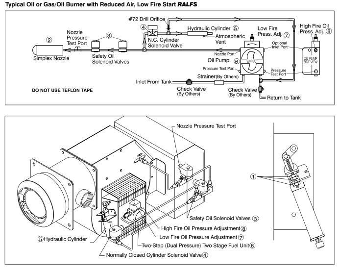
MECHANICAL OPERATION: The RALFS system uses a two step, two stage dual pressure Oil Pump (6), or fuel unit, with a simplex nozzle. Either a direct spark or a gas pilot ignition system may be provided for ignition of the main oil flame. The air damper is spring loaded to an open position suitable for maximum desired capacity and proper combustion.
