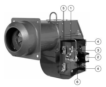
MECHANICAL OPERATION: The On-Off system uses a single stage, high suction lift Oil Pump (2) with a Simplex Oil Nozzle. A direct spark oil ignition system is standard on typical oil burners (a gas pilot is standard on Gas/Oil burners), but certain insurance company codes could
