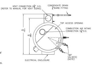
Note: The standard temperature and relief valve meet ASME/CSA Ratings. Models up to 600 MBH will have one relief valve, models 700 MBH and above will have two.
