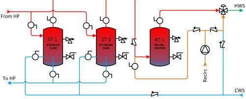
**Multi-pass** heat pump example configuration with recirculation
