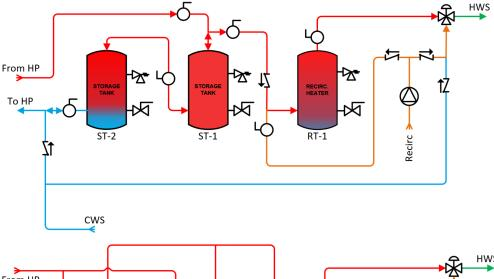
**Single-pass** heat pump example configuration with recirculation
