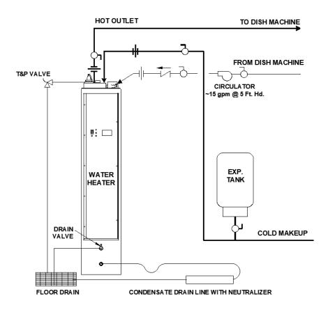
Figure 4-4: Configuration for Dish Washing Application
