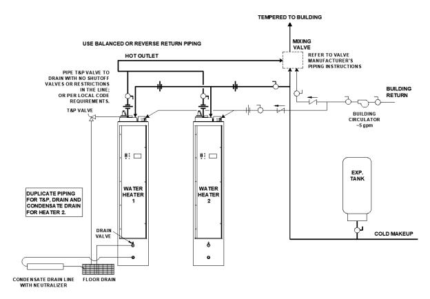
Figure 4-3: Two Water Heaters with Reverse Return Piping
