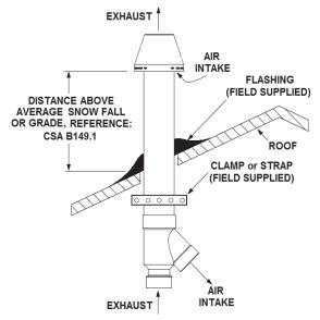
Figure 8-1: Roof Termination
