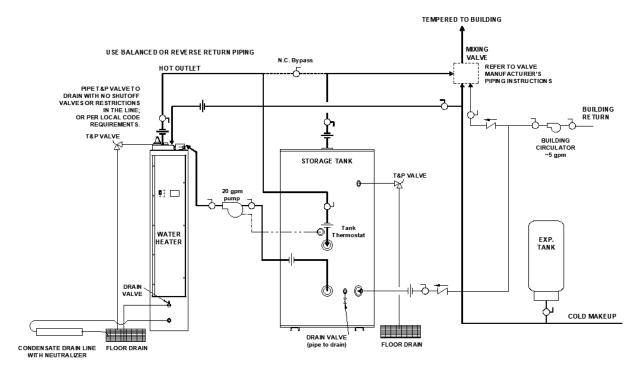
Figure 4-2: Single Water Heater with Supplemental Storage Tank
