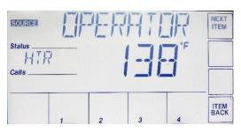
All heaters are factory set to 120F. if replacing a PIM module in the field, this must be adjusted.
