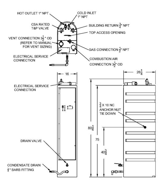
Figure 2-1: Component, Controls and Connection Locations
